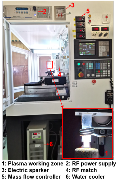
Fig. 1. Atmospheric ICP setup.
